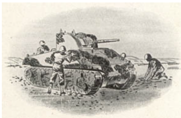
FIGURE 37. Thick mud being applied in a disruptive pattern to a tank.
